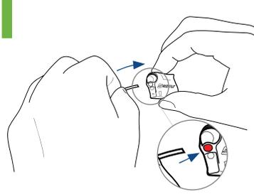
Insert the cable into the middle hole.
