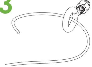
Loop cable around or through structural mounting points. Examples of mounting points: eye-bolts, ceiling trusses, I-beams, unistrut, etc.
