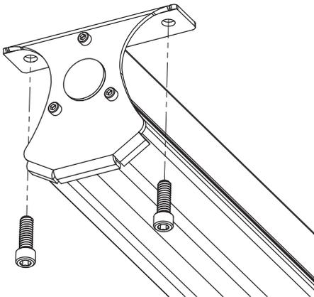
Mount bracket to the structure or wall. Hardware to mount bracket to structure is not provided. Ensure mounting surface is able to support weight of fixture.
