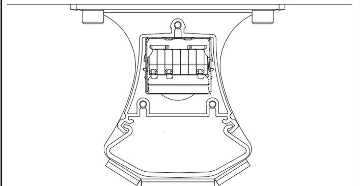
Ensure the fixture is firmly mounted with the brackets flush to mounting surface and all hardware flush to the mounting bracket.
