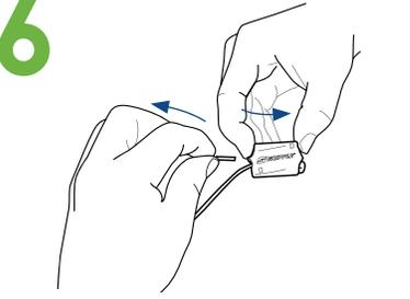
While the button is pressed, adjust the cable. When the desired position is reached, release the button to lock.
