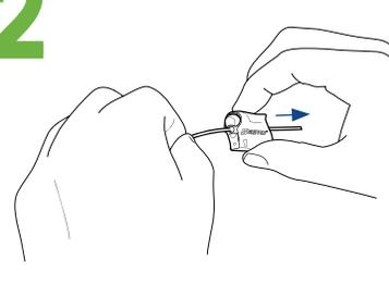
Slide the grip lock along the cable and loop through the top mounting point.
