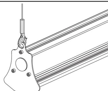
Snap hooks through mounting holes in endcaps.
