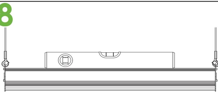
Ensure the fixture is level before proceeding to electrical connections.
