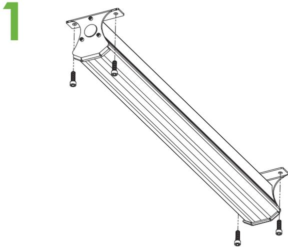
Fixtures ship with pre-installed surface mount brackets. Each endcap has (3) 1/4" mounting holes, see "2" for bracket hole pattern.
