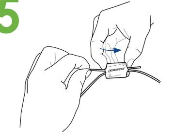
Release the load of the quick-lock and push the release button in the same direction of the wire entrance.
